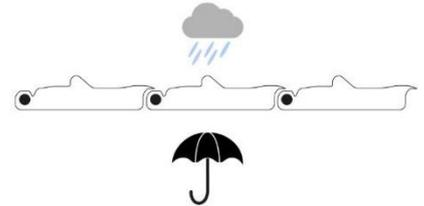
The bioclimatic blades are directional shutters that allow you to adjust the amount of sunlight to your terrace to climatic conditions or as desired.
